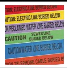
**Non-Detectable Underground Warning Tape** - Acts as a safety warning against inadvertent intrusion in the cable right of way. The warning tapes are treated so as not to degrade or fade when exposed to alkalis, acids and/or other destructive elements underground. All tapes are made of tough virgin polyethylene materials.
